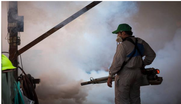
Thermal Hot Fogger Treatment
